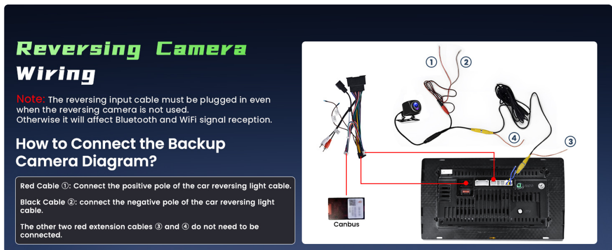
Figure 16: Wiring diagram for the reversing camera.
