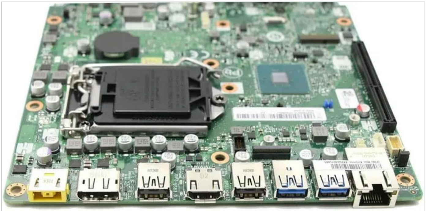
Figure 3.1: Generic Motherboard Model 8012111968584. This image displays the Generic Motherboard, model 8012111968584. Visible components include the CPU socket, two DDR4 memory slots, multiple USB ports (both USB 2.0 and USB 3.0), an Ethernet port, and other integrated circuits. The board features a green PCB and standard component layout.
