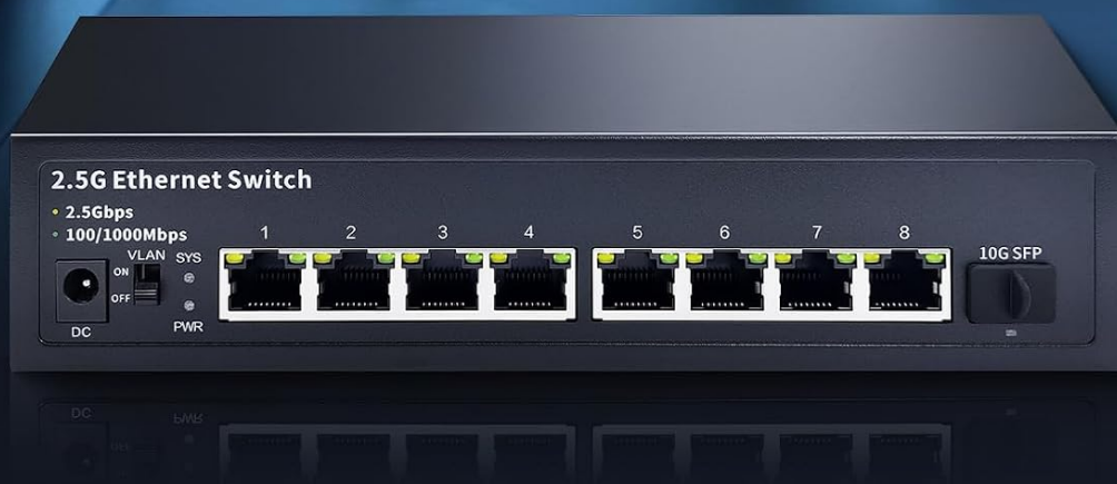
Image 6.1: Close-up view of the VLAN toggle switch, showing 'ON' and 'OFF' positions.
