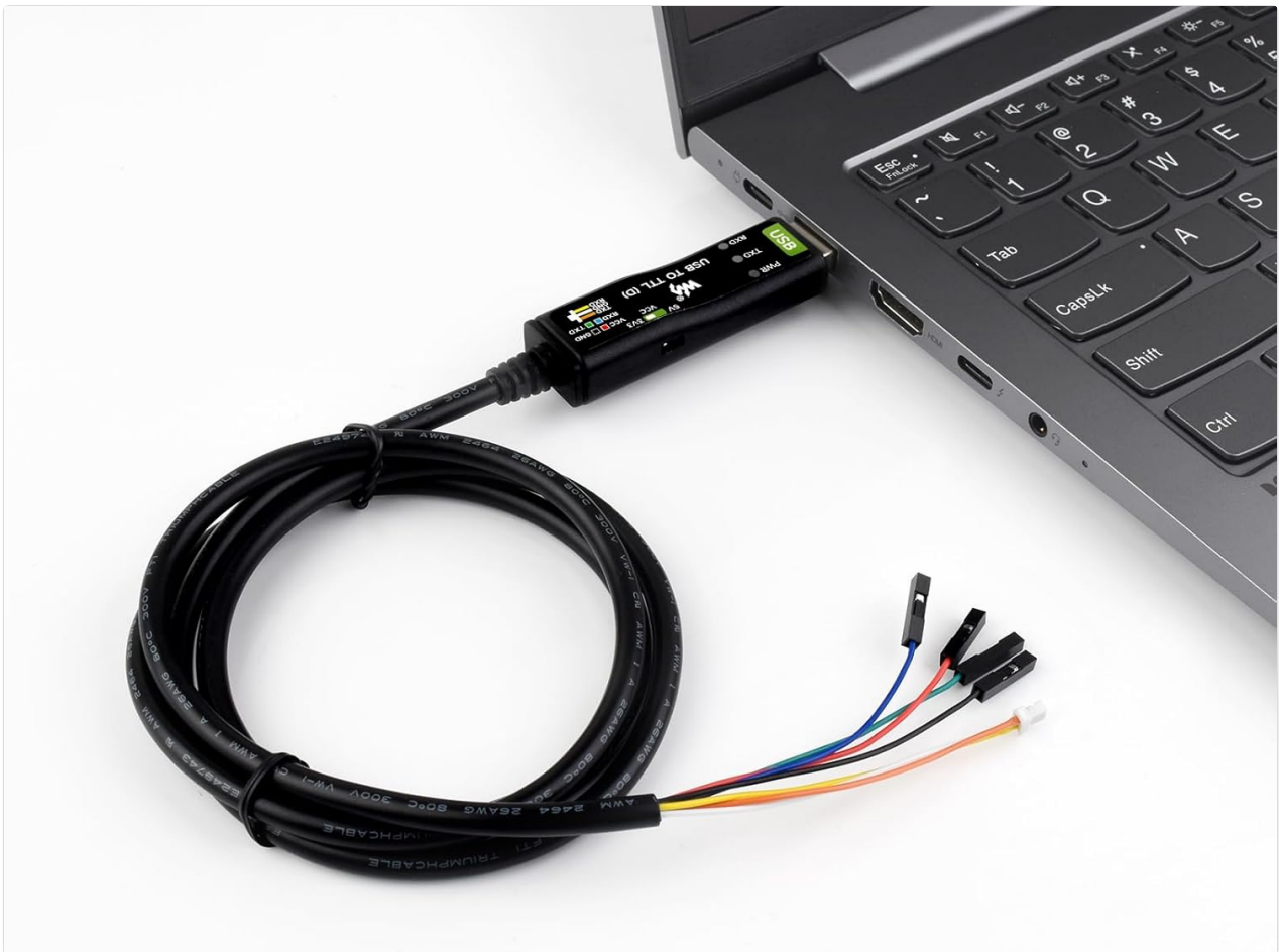
Image 5: The waveshare USB to TTL adapter connected to a laptop, demonstrating a typical usage scenario.
