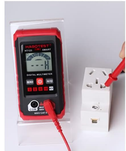
Neutral line and live line measurement
