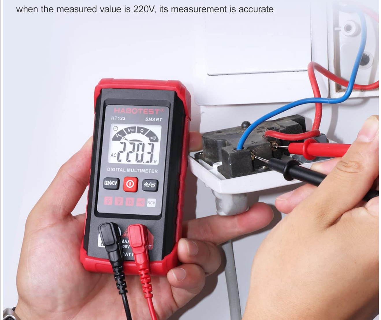
Image 6.2: The HT123 Multimeter measuring AC voltage from a wall outlet, displaying a reading of 220.3V.
