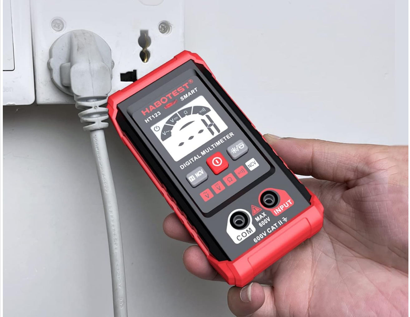
Image 6.3: The HT123 Multimeter performing non-contact voltage detection near a wall outlet, indicated by the NCV icon and signal strength bars on the display.
