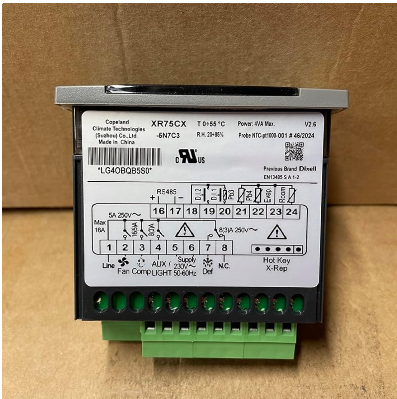
Image 4.1: Rear view of the XR75CX-5N7C3 thermostat, illustrating the screw terminal block and integrated wiring diagram for power, probes, and relay outputs.
