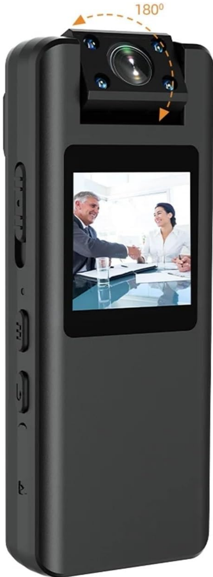
Image 2.2: The VCHICS A22 Mini Body Camera demonstrating its 180-degree rotatable camera head for flexible recording
