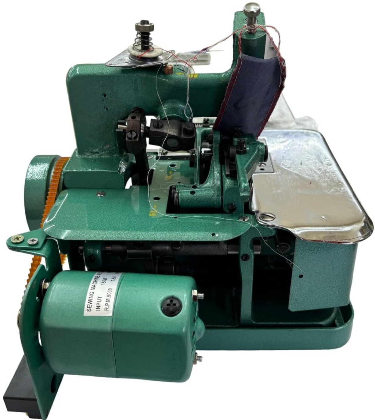
Figure 6: Alternate side view, providing a closer look at the motor and drive belt.
