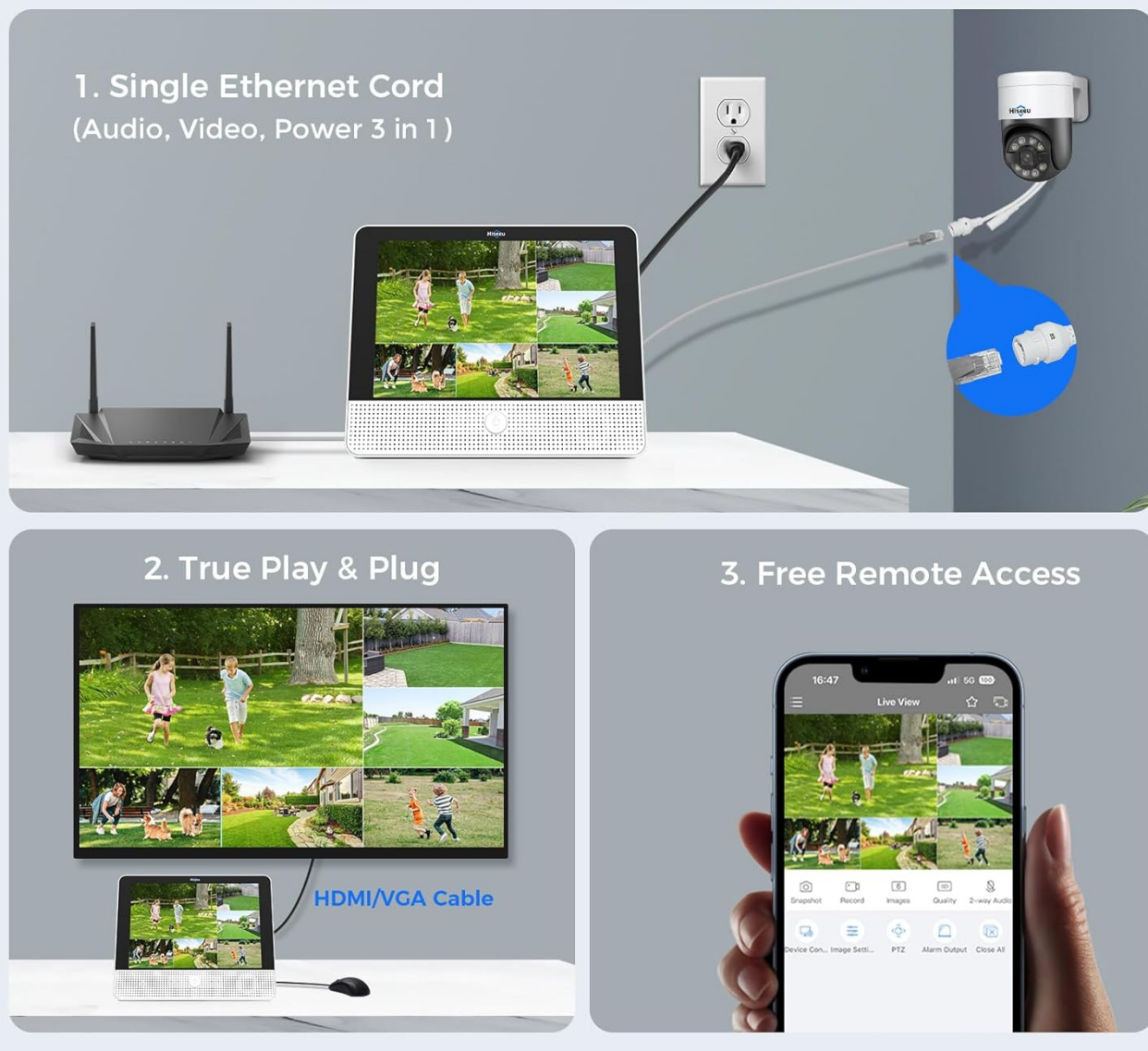
Figure 3.1: Illustration of the Power over Ethernet (PoE) connection for cameras and options for local and remote viewing.
