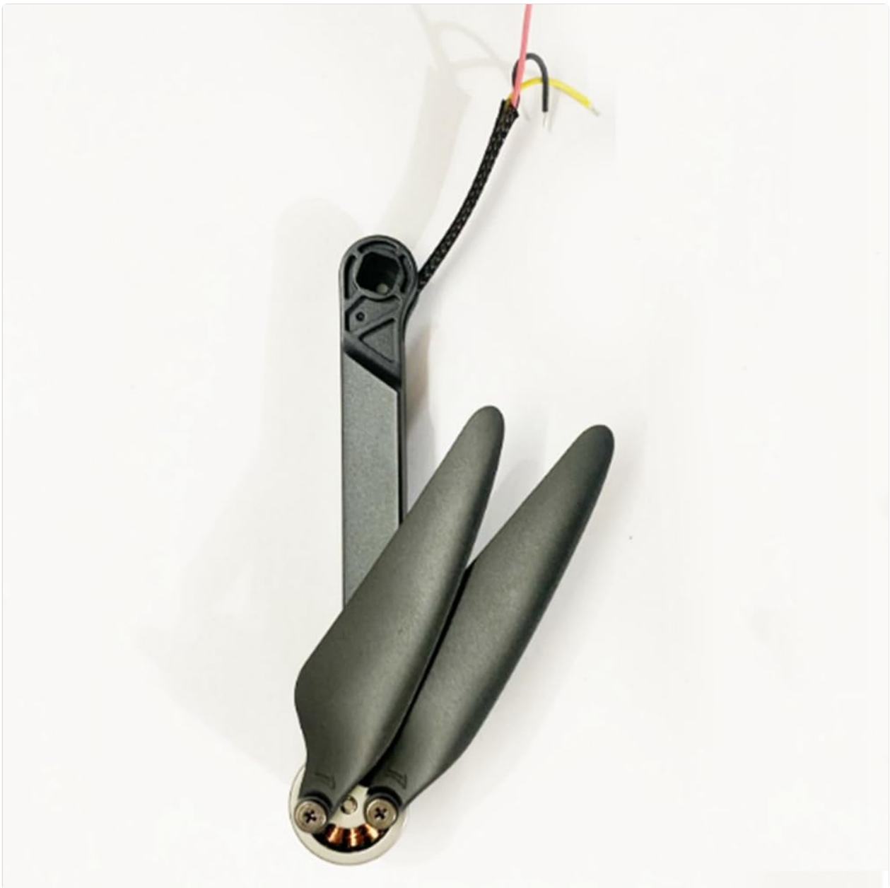
Figure 2: A folded view of the TSPFJX Rear A Arm, showing the compact design and the wiring harness extending from the base. This perspective helps in understanding the arm's articulation.
