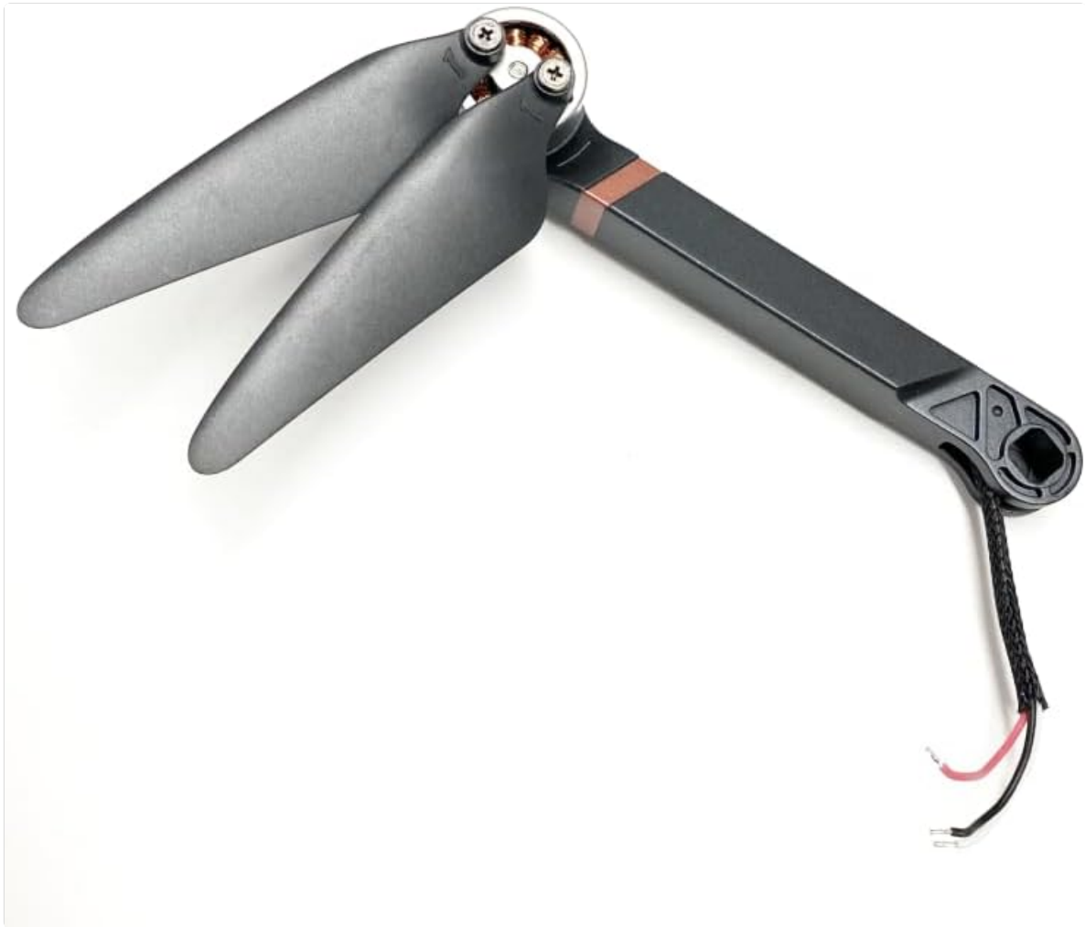
Figure 1: The TSPFJX Rear A Arm with integrated motor and propellers. This image shows the complete assembly ready for installation, highlighting the motor, propeller blades, and wiring.
