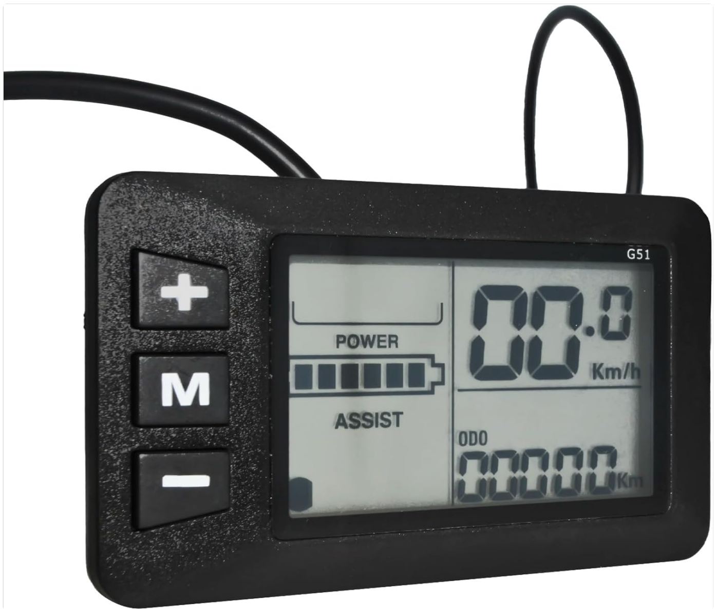
Figure 3.1: A detailed view of the G51 display, highlighting the '+', 'M', and '-' buttons on the left side, and the various data fields on the screen.
