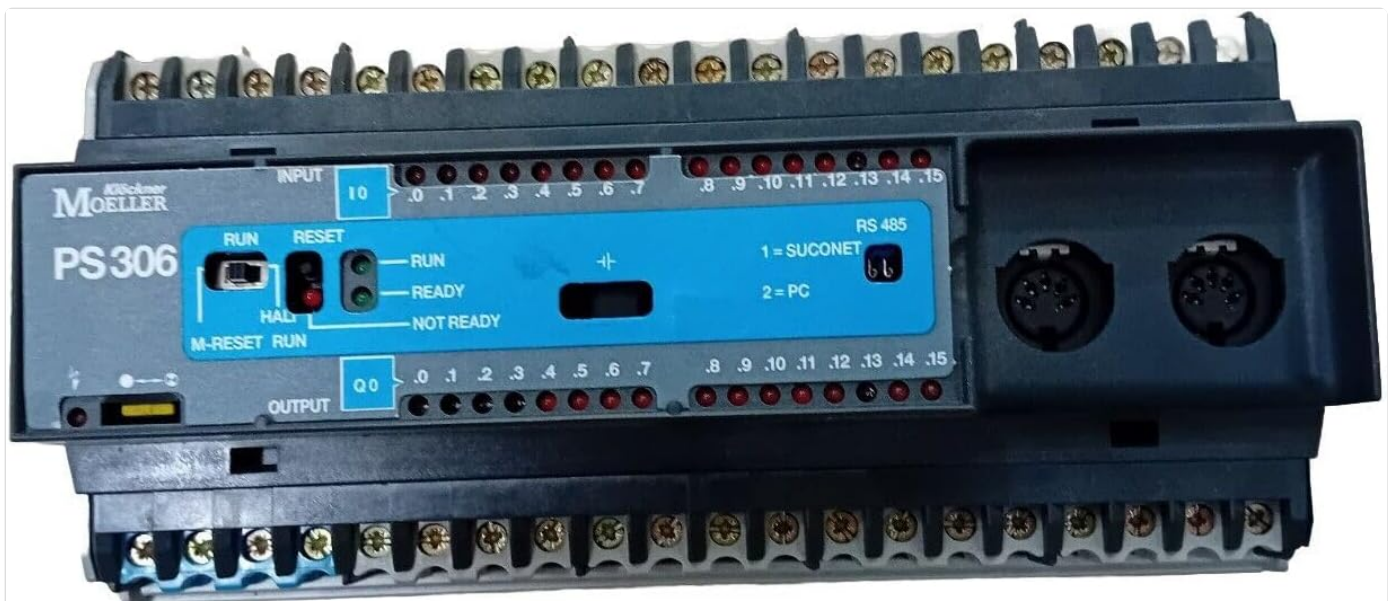
Figure 1: Front view of the MOELLER PS306-DC-EE PLC, showing input/output terminals, status LEDs, and communication ports.
