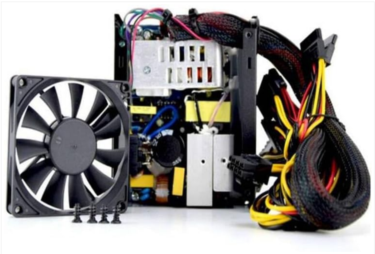
Figure 4.1: Internal view of the SFX-500W power supply, highlighting the cooling fan and internal circuitry.
