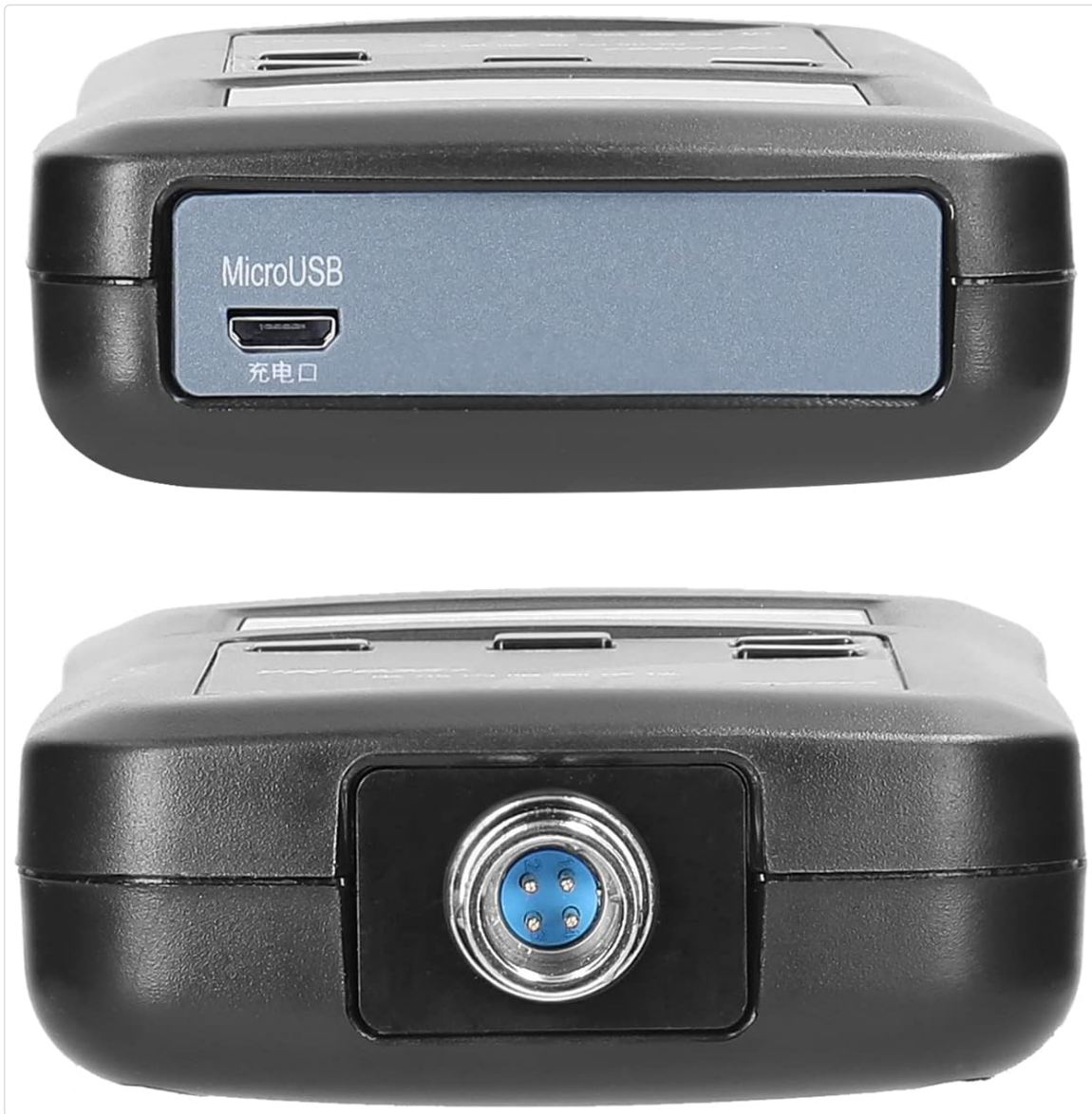
Figure 4.2: Top and bottom view of the YR1035+ tester, showing the MicroUSB charging port and the dedicated port for connecting the test probes.
