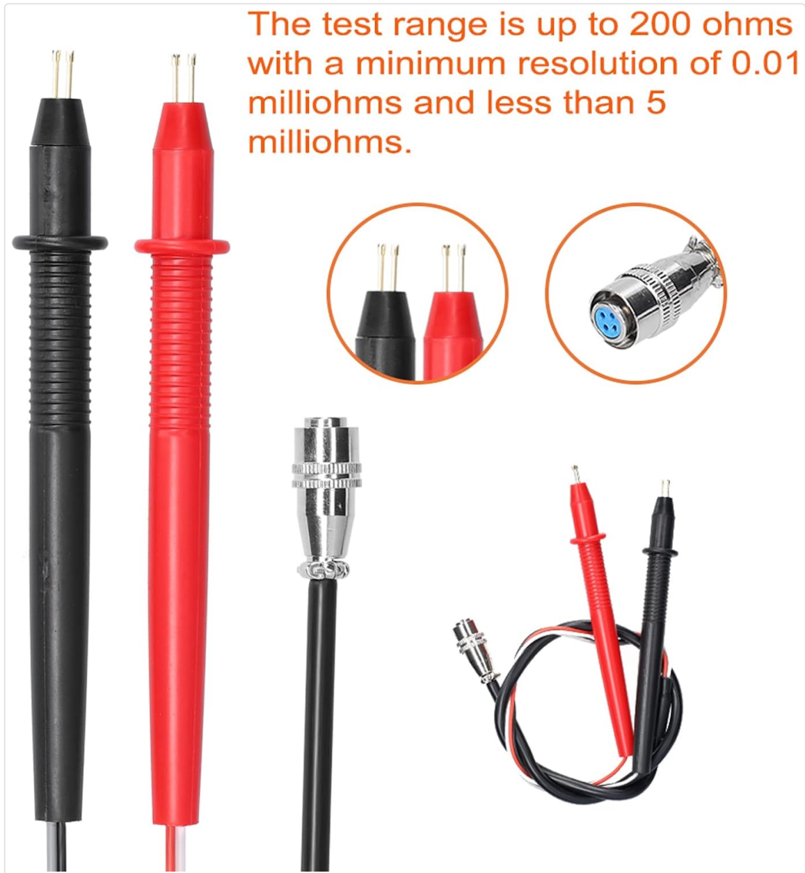
Figure 5.1: The set of test probes included with the YR1035+ tester, designed for 4-wire measurements.
