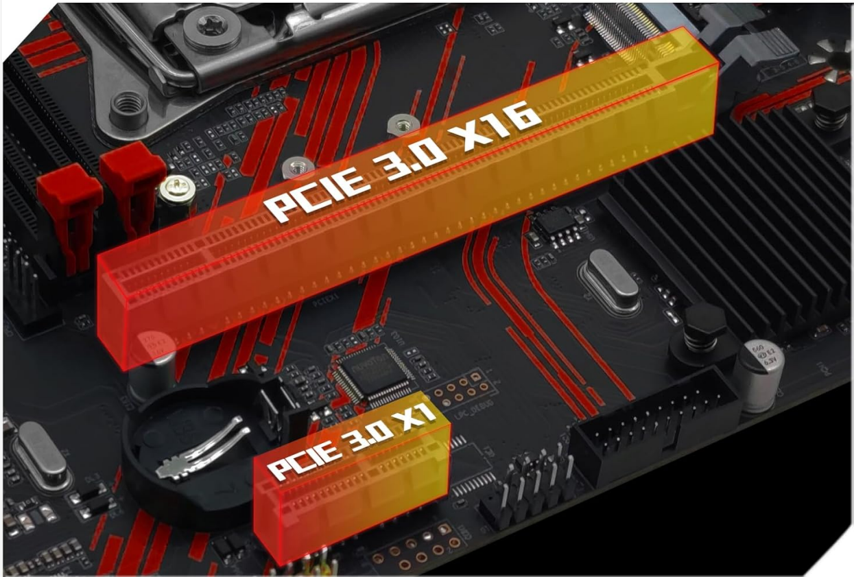
Image: Close-up of the PCIe 3.0 x16 and PCIe 3.0 x1 expansion slots on the motherboard, indicating their positions.
