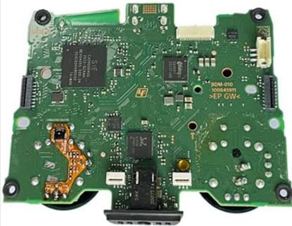
Calibration PCB with MCU stacks on the main PCB
