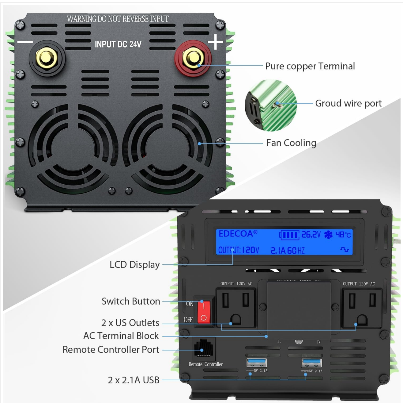
Image: The rear panel of the EDECOA 3000W Power Inverter, displaying the positive (red) and negative (black) DC input terminals, dual cooling fans, and a ground wire port.
