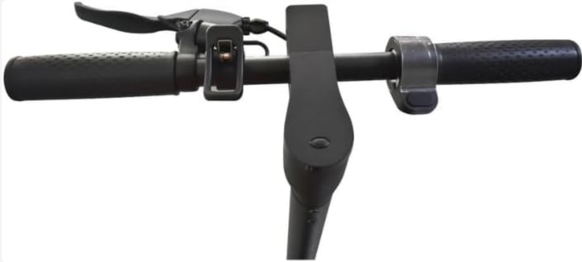
Figure 5.1: Detailed view of the handlebar, showing the accelerator, brake lever, and control panel.
