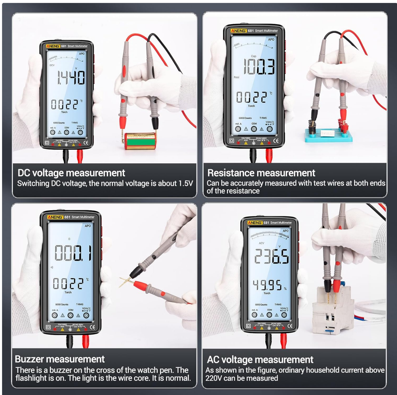
Figure 6.1: Demonstrations of various measurement functions: DC voltage measurement (top left), Resistance measurement (top right), Buzzer continuity test (bottom left), and AC voltage measurement (bottom right).
