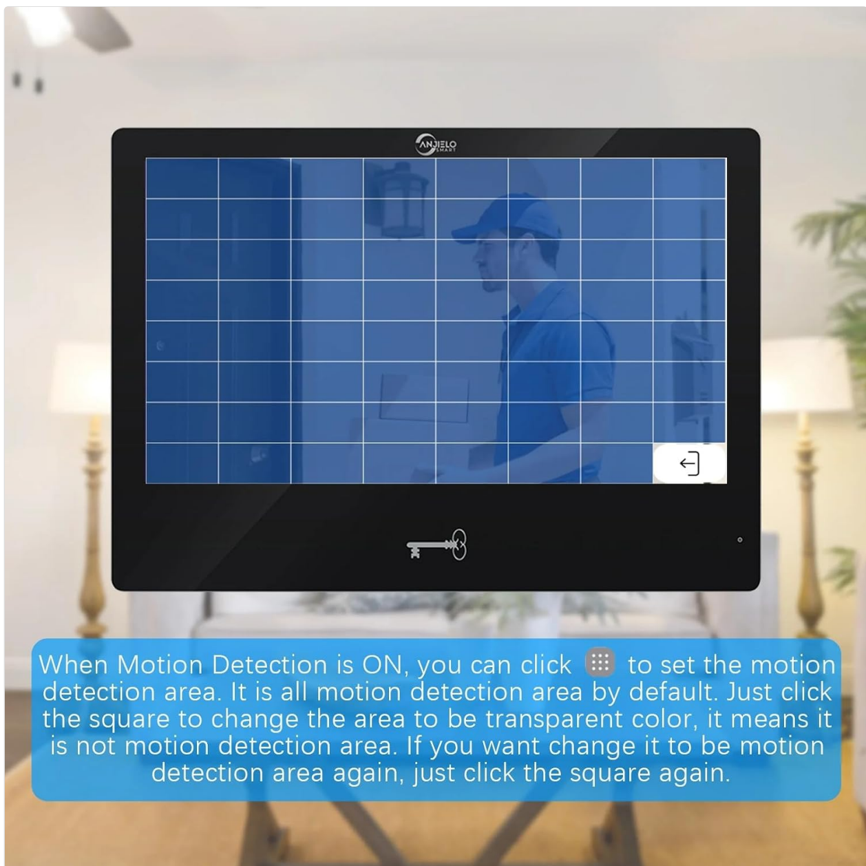
Figure 4.5: Instructions on how to customize the motion detection area on the indoor monitor by selecting or deselecting grid squares.
