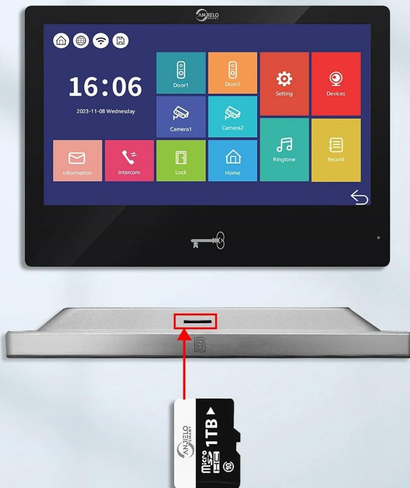
Figure 4.7: Location of the SD card slot on the indoor monitor for recording events.
