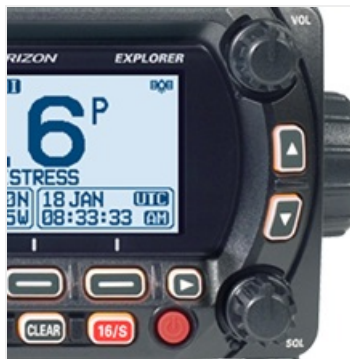
Image: Close-up of the volume and squelch control knobs on the GX1800G.
