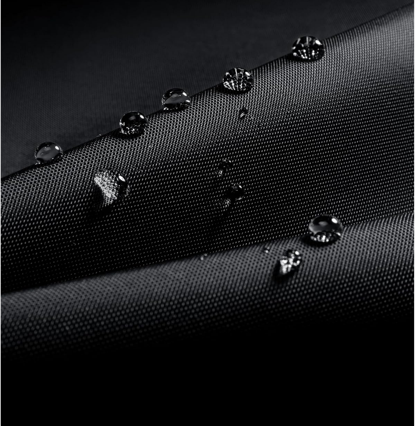
Image 4.1: Close-up of the Cordura 420D Nylon fabric, demonstrating its water-resistant properties.
