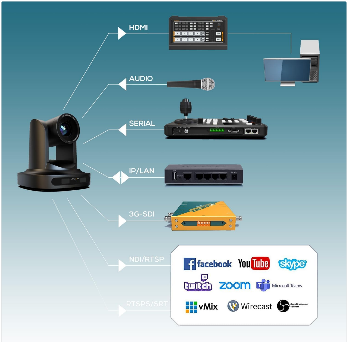
Figure 3.3.1: Connectivity Diagram of AVIDEONE PTZ Camera. This diagram illustrates the various input and output ports on the camera's rear panel, including HDMI, 3G-SDI, LAN (PoE), RS232/RS485, and audio input, along with examples of connected devices and streaming platforms.
