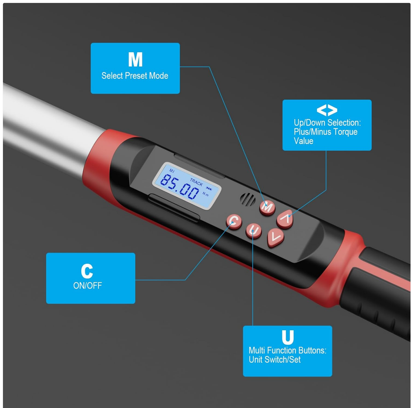
Figure 2.2: Detailed view of the control panel with M (Select Preset Mode), C (ON/OFF), U (Multi Function Buttons: Unit Switch/Set), and Up/Down arrows (Plus/Minus Torque Value).
