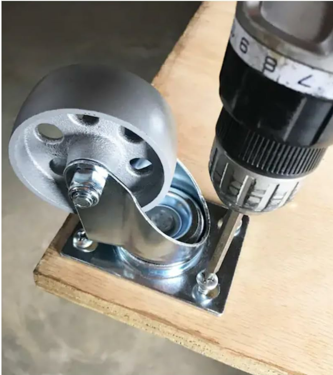
Image 4.1: Caster Installation Example. This image shows a caster being mounted to a wooden surface using a drill and screws, demonstrating the typical installation process.
