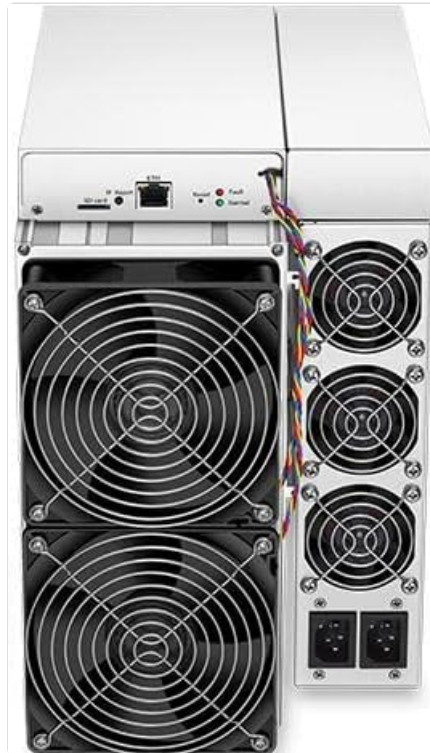
Figure 4.1: Top-down view of the Antminer KS5 Pro's control board, showing the Ethernet port, IP Report button, and status indicator LEDs (Fault, Normal).
