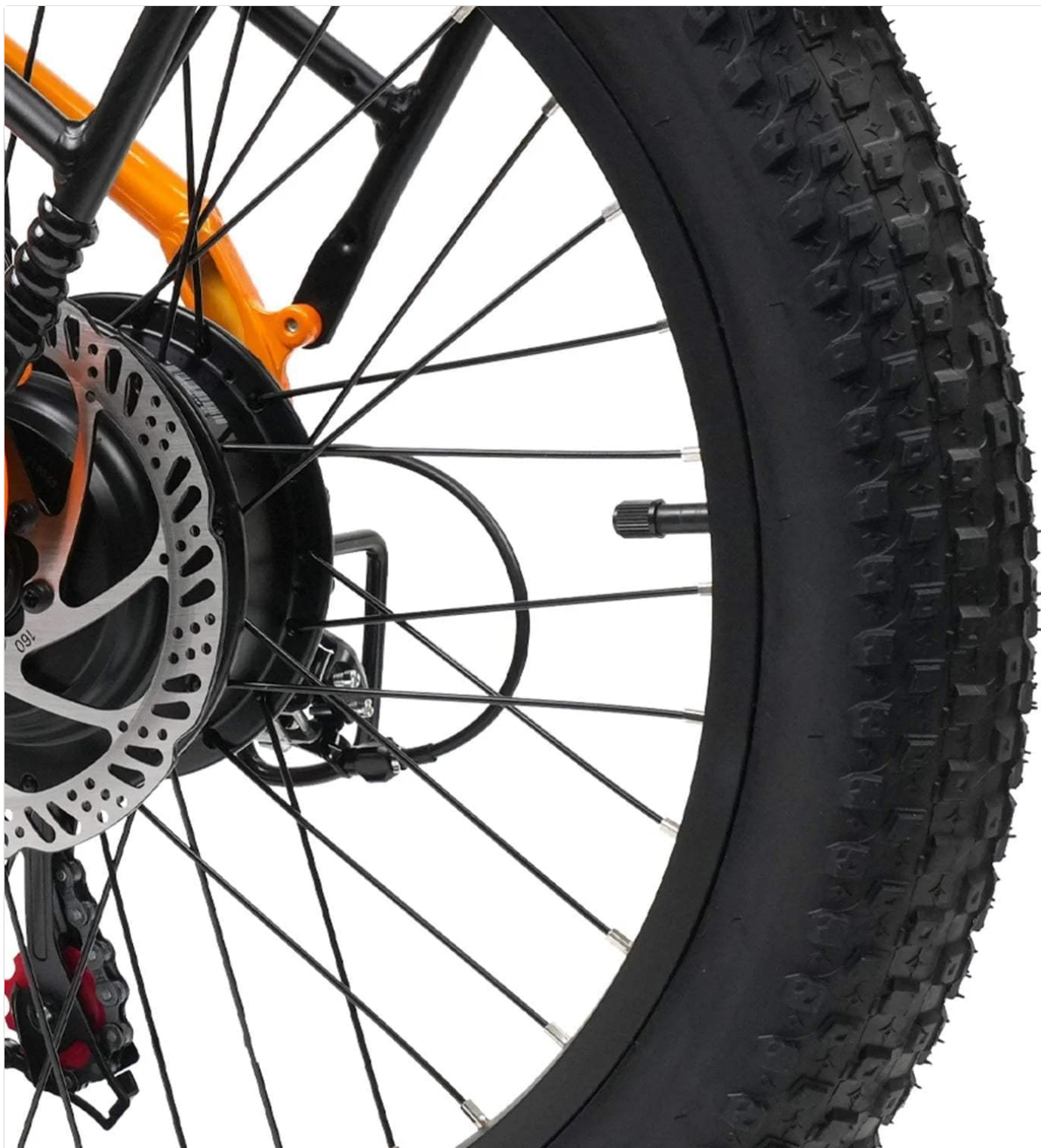
Figure 4.2: Close-up view of the rear disc brake system, providing consistent braking performance.
