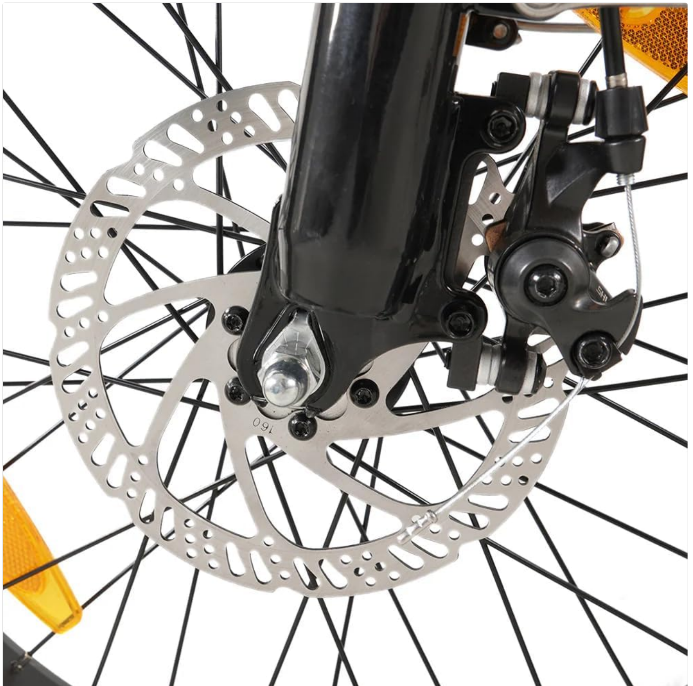
Figure 4.1: Close-up view of the front disc brake system, ensuring reliable stopping power.
