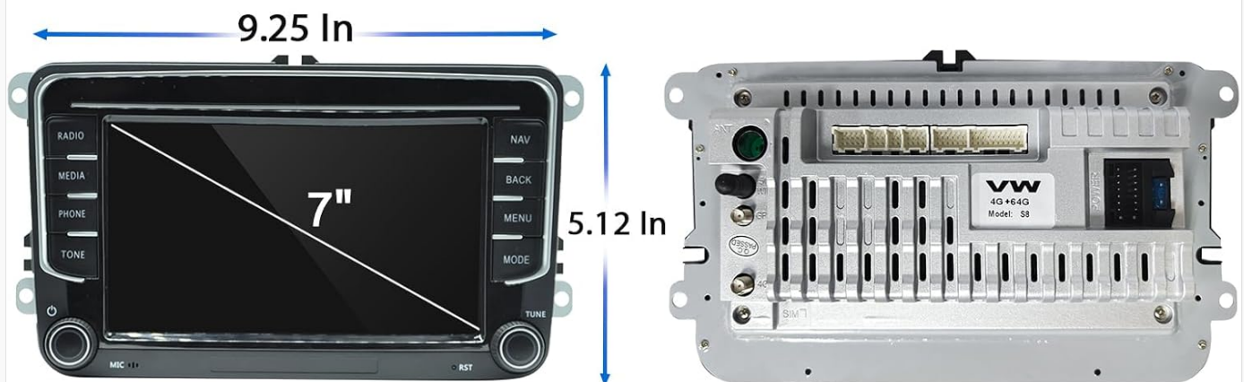
Figure 4.1: Wiring Connections and Product Dimensions
