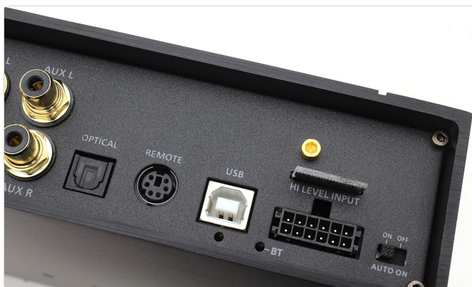
Figure 2.3: Detailed view of the input section, including RCA, Optical, Remote, USB, and High-Level Input ports.
