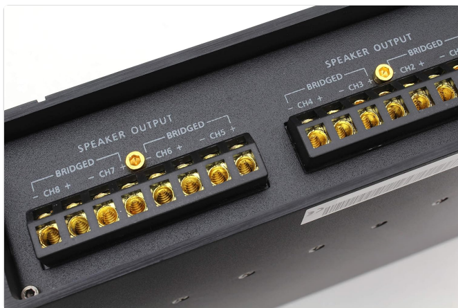
Figure 2.4: Close-up of the speaker output terminals, clearly labeled for individual channels and bridged configurations.
