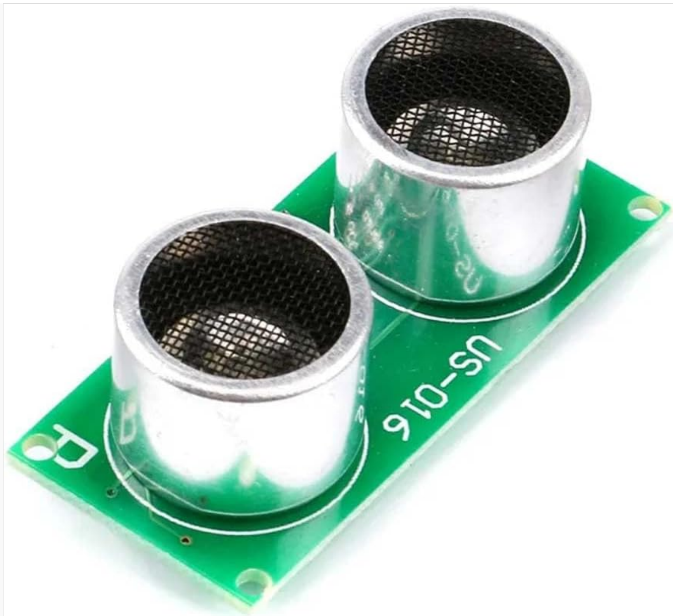
Figure 1: Angled view of the US-016 module, showing the two ultrasonic transducers.
