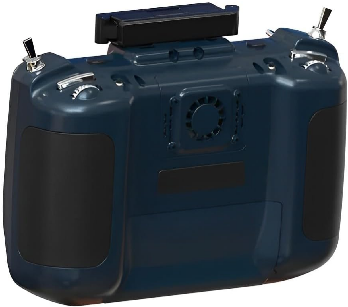
Image: Rear view of the Jumper T20S V2 Radio Controller, displaying the external cooling fan and battery compartment area.
