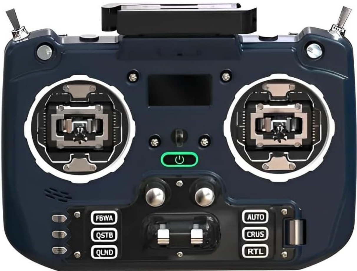
Image: Angled front view of the Jumper T20S V2 Radio Controller, highlighting the gimbals and control layout.
