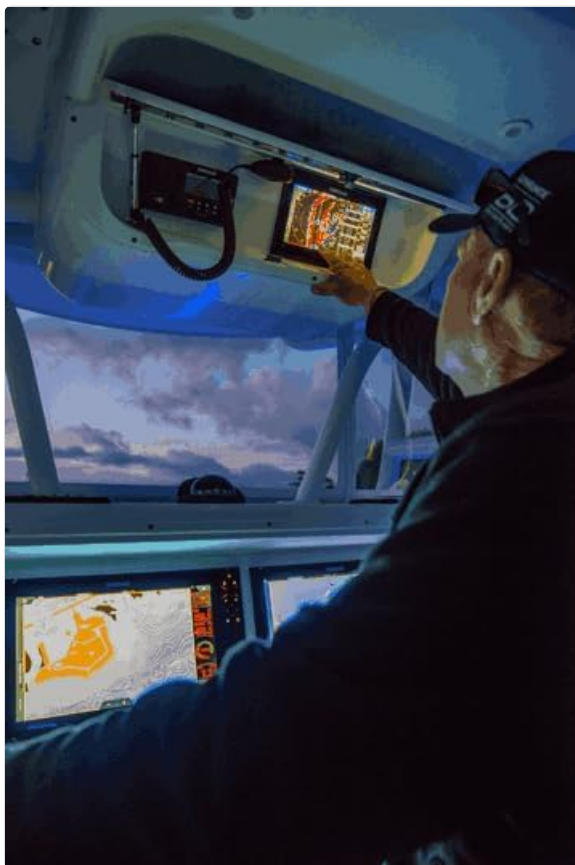
Figure 3.1: The Simrad GO9 XSE displaying a detailed navigation chart with route information and current vessel data.
