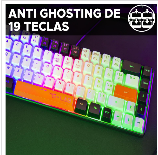
Image 2.4: 19-Key Anti-Ghosting. This technology ensures that up to 19 keys can be pressed simultaneously without any input conflicts, crucial for complex gaming commands.
