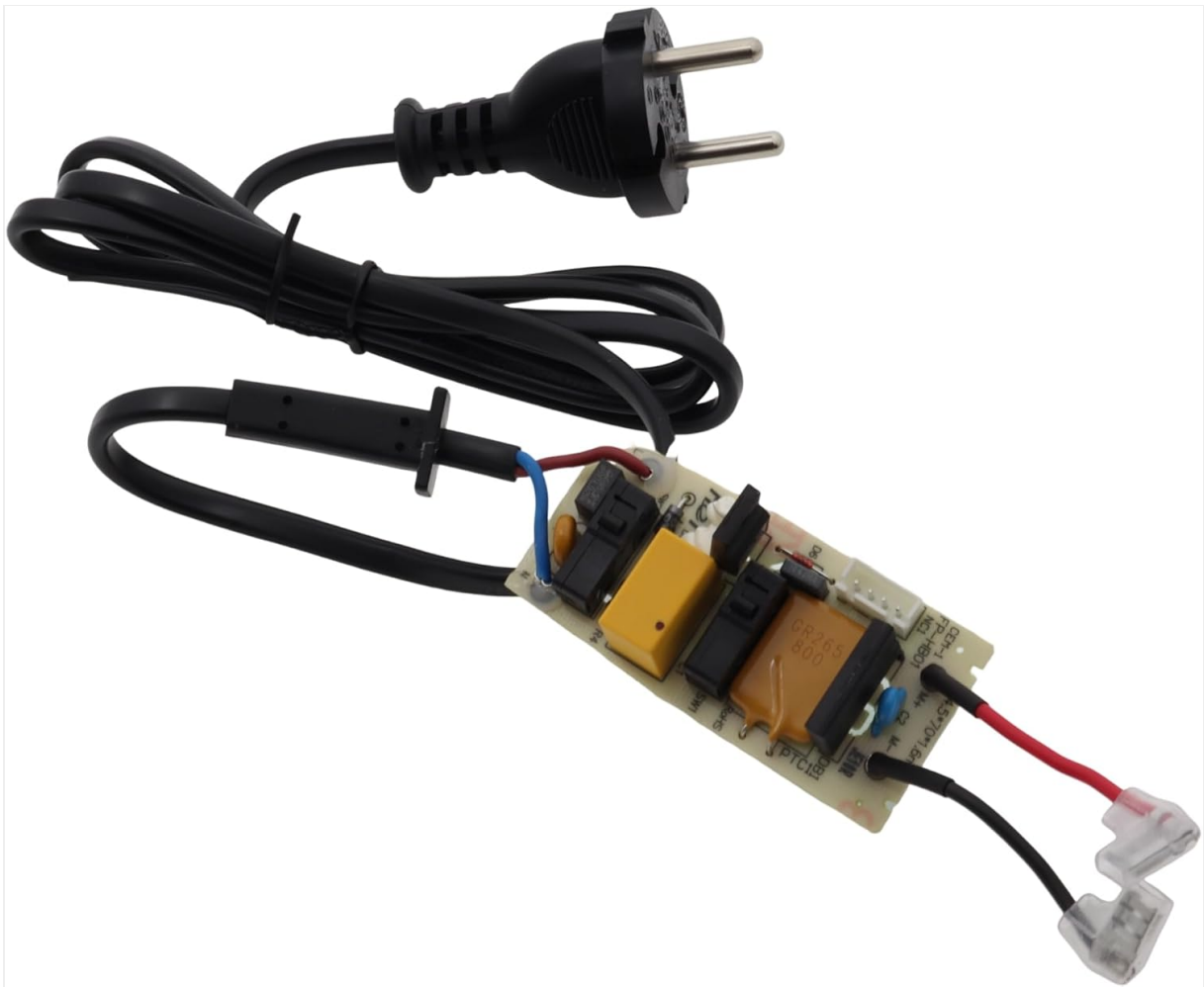
Image 3: Moulinex PCB and power cable with EU plug, showing reverse side with larger components. This perspective reveals the underside of the PCB, including larger capacitors and other power regulation components.
