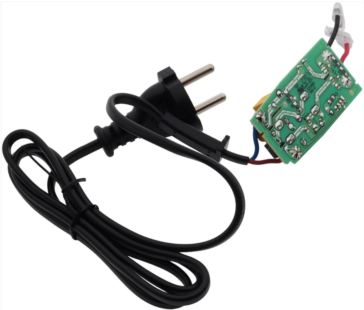
Image 2: Moulinex PCB and power cable with EU plug, showing component side. This view highlights the various electronic components mounted on the circuit board, essential for the blender's operation.
