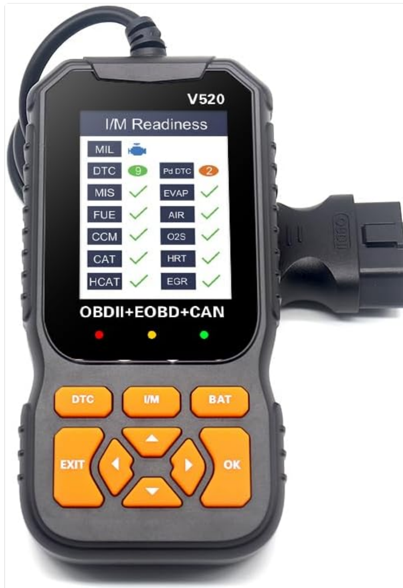
Figure 5: The V520 displaying the I/M Readiness status. This screen shows the completion status of various emission-related monitors, such as MIL (Malfunction Indicator Lamp), DTC (Diagnostic Trouble Codes), MIS (Misfire Monitoring), FUE (Fuel System Monitoring), CCM (Comprehensive Component Monitoring), CAT (Catalyst Monitoring), HCAT (Heated Catalyst Monitoring), AIR (Secondary Air System Monitoring), EVAP (Evaporative System Monitoring), O2S (Oxygen Sensor Monitoring), and EGR (Exhaust Gas Recirculation System Monitoring).
