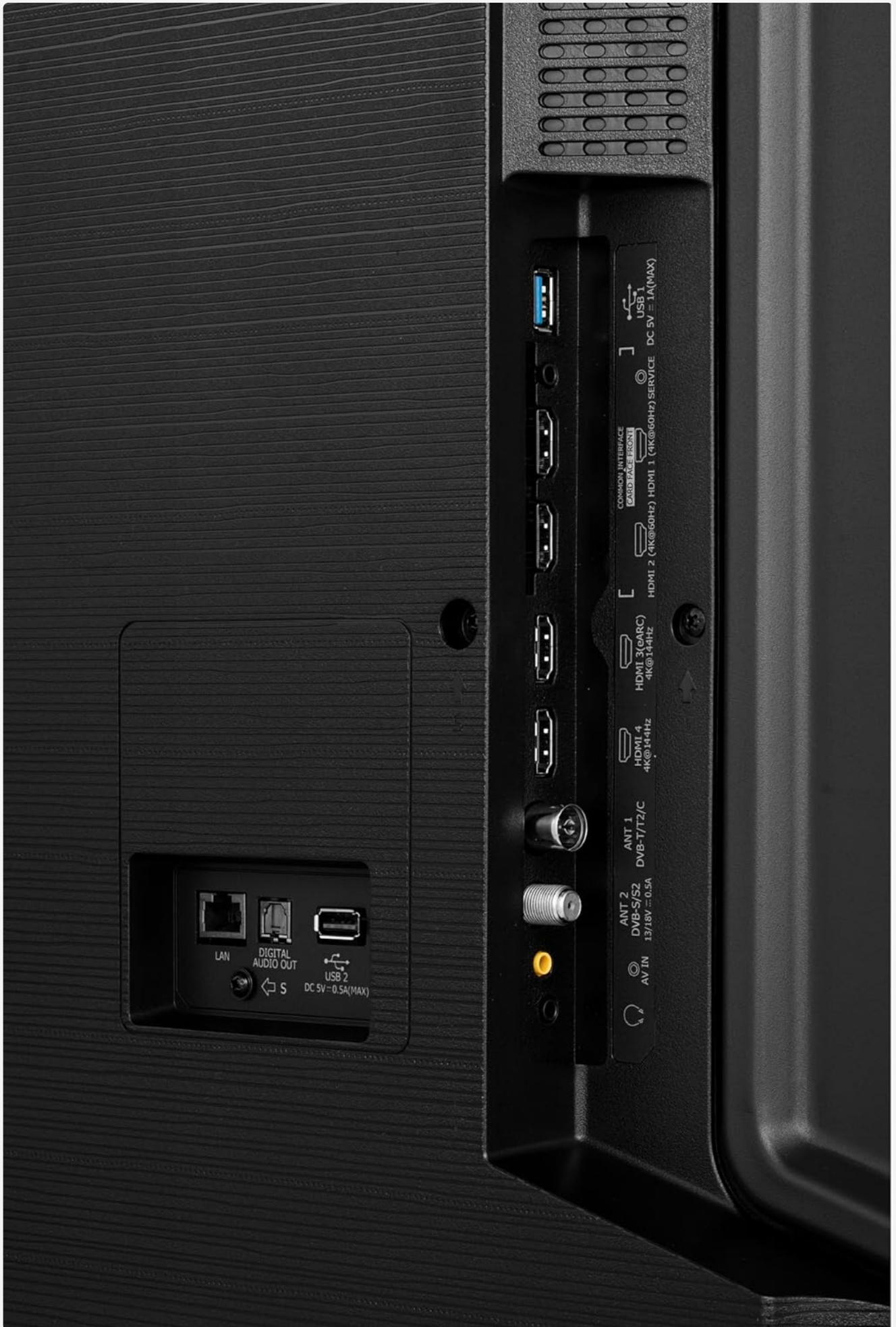
Detailed close-up of the connectivity ports on the back of the Hisense 75U7NQ TV, including HDMI, USB, LAN, and antenna inputs.
