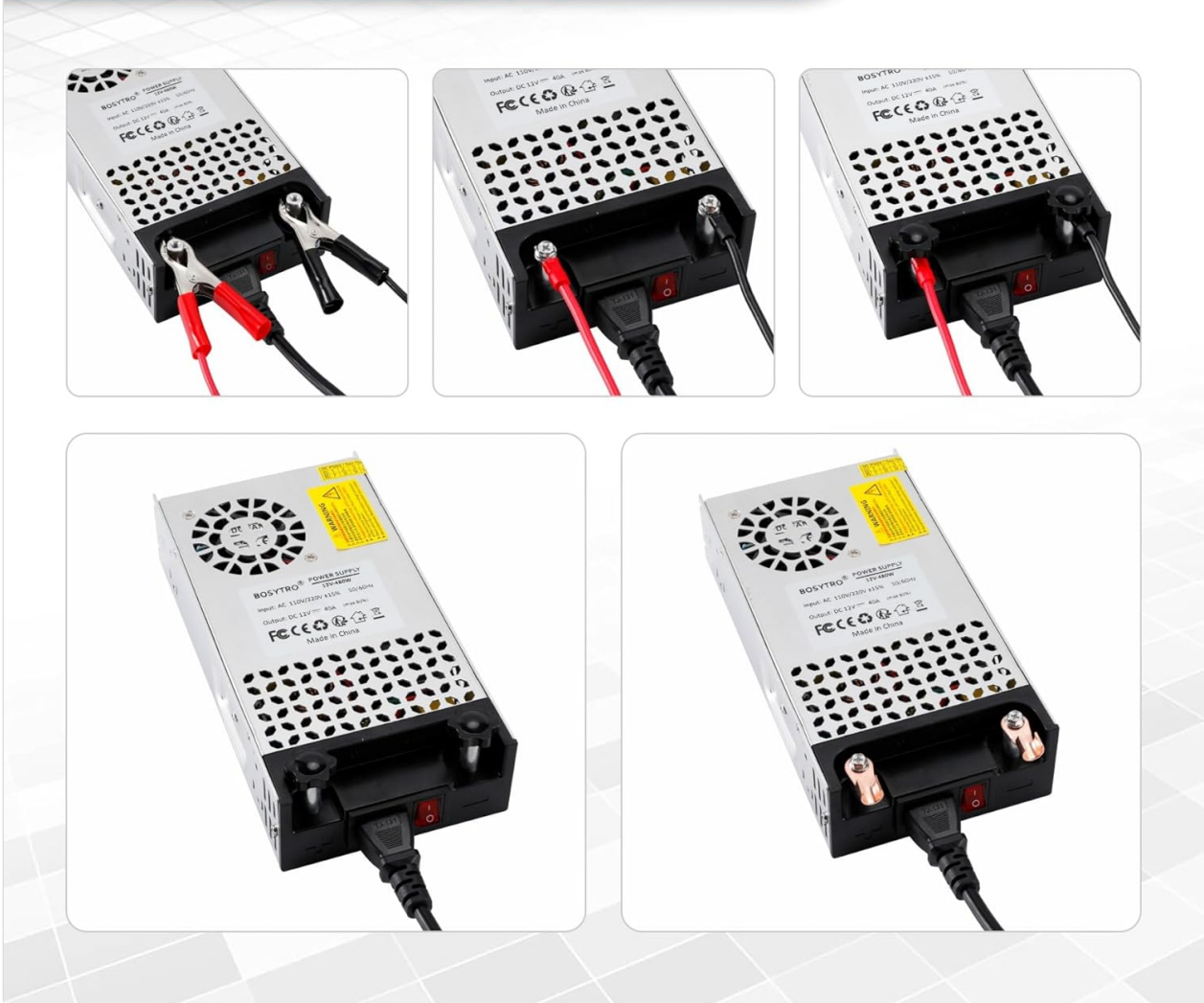
Image 3.3: Examples of connecting devices to the power supply using alligator clips, bare wires, or ring terminals. Always ensure secure and correct polarity connections.
