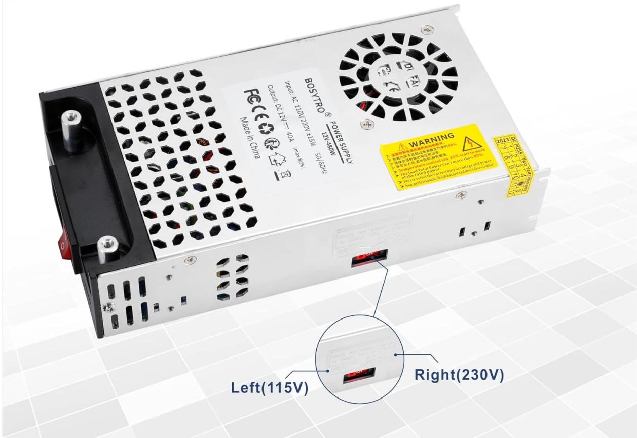
Image 3.2: The input voltage selector switch, showing positions for 115V (left) and 230V (right). Ensure this is set correctly for your local power grid.
