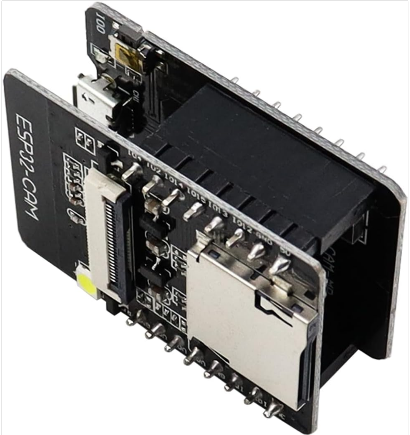
Image 5.1: Angled view of the ESP32-CAM module, illustrating the micro USB port for power and data, and the accessible pin headers.
