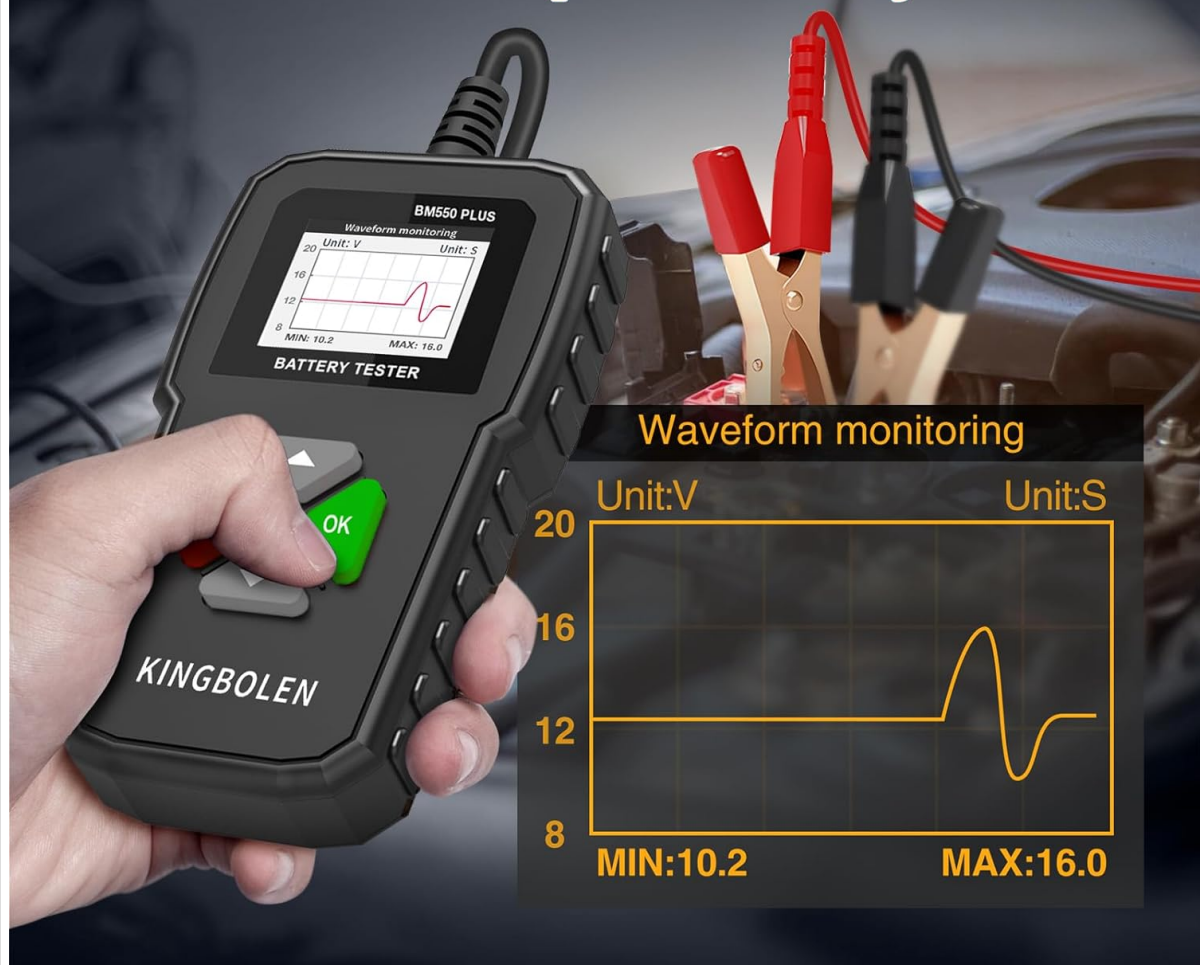
Image 6.3: The BM550 Plus monitoring real-time voltage waveforms.
