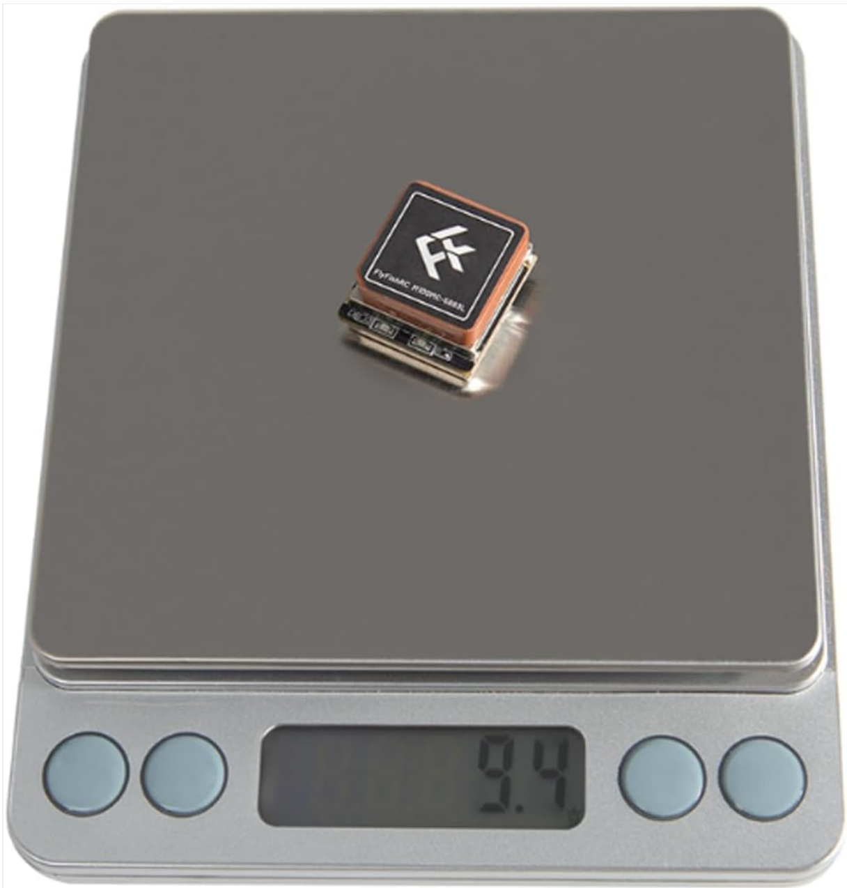
Figure 7.2: Weight of the FlyFishRC M10QMC-5-8-83L GPS Module. The module is shown on a digital scale displaying a weight of 9.4 grams.
