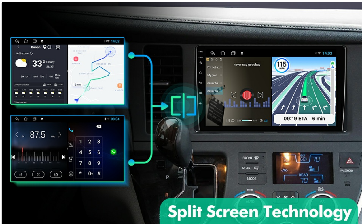
Figure 8: The car stereo display demonstrating split-screen functionality, showing navigation on one side and music controls on the other.
