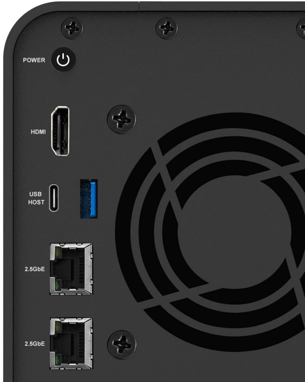
Figure 6: Rear panel connectivity of the F2-424 NAS.
