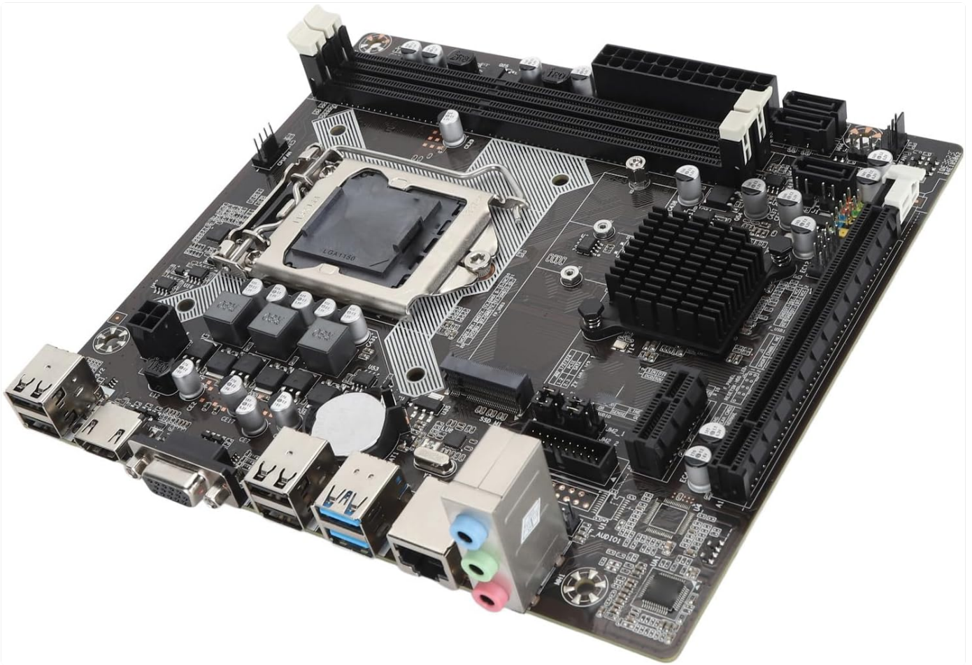
Figure 3.3: Rear I/O panel with USB, VGA, HD Multimedia Interface, LAN, and audio ports.
