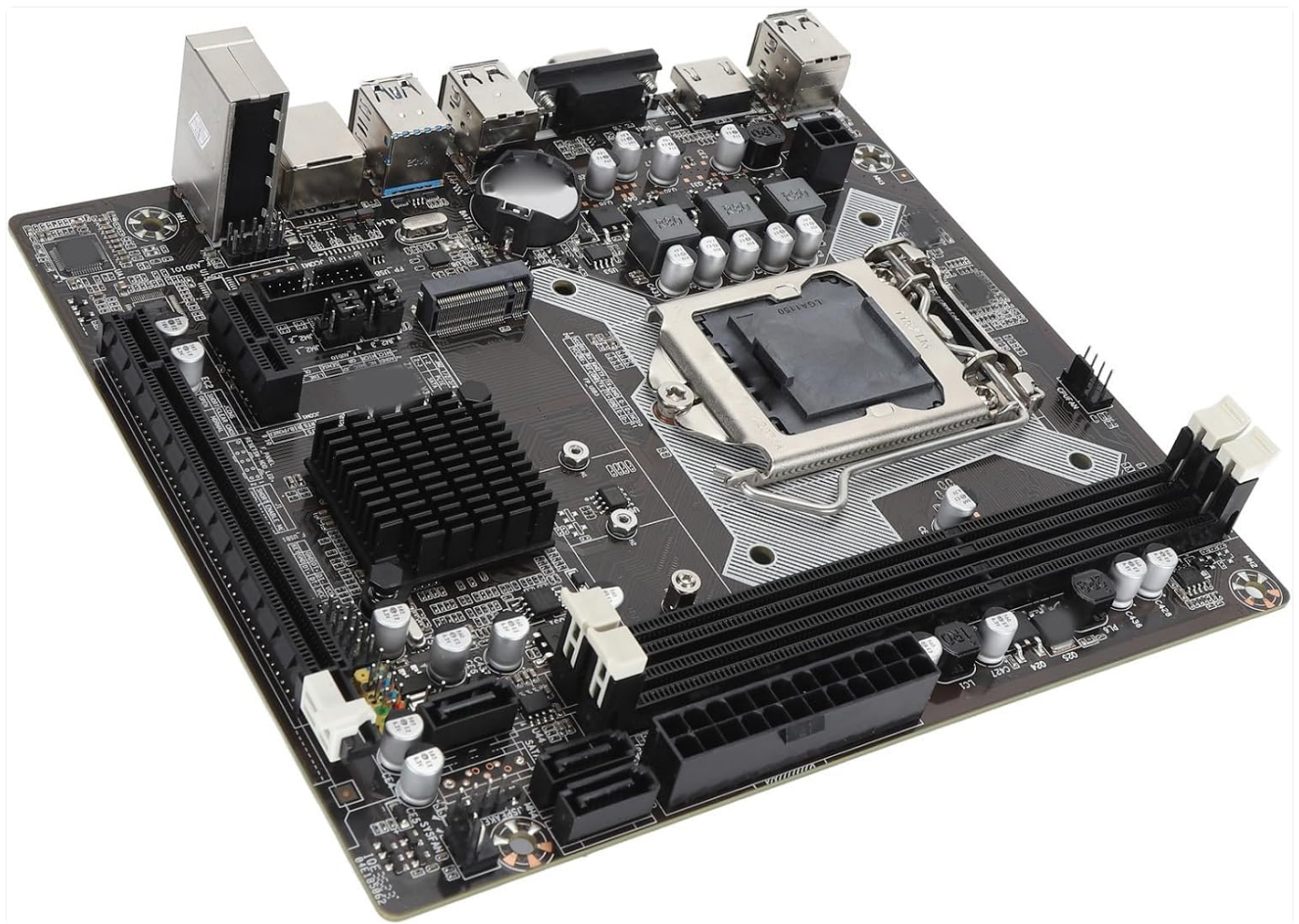
Figure 3.2: The two DDR3 DIMM slots and the 24-pin ATX power connector.
