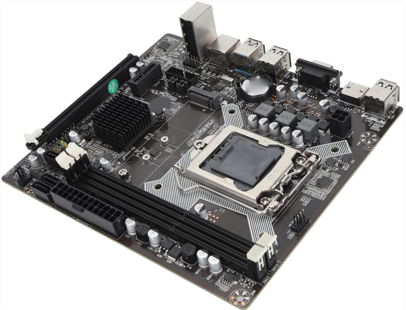
Figure 3.1: The LGA1150 CPU socket, ready for processor installation.
