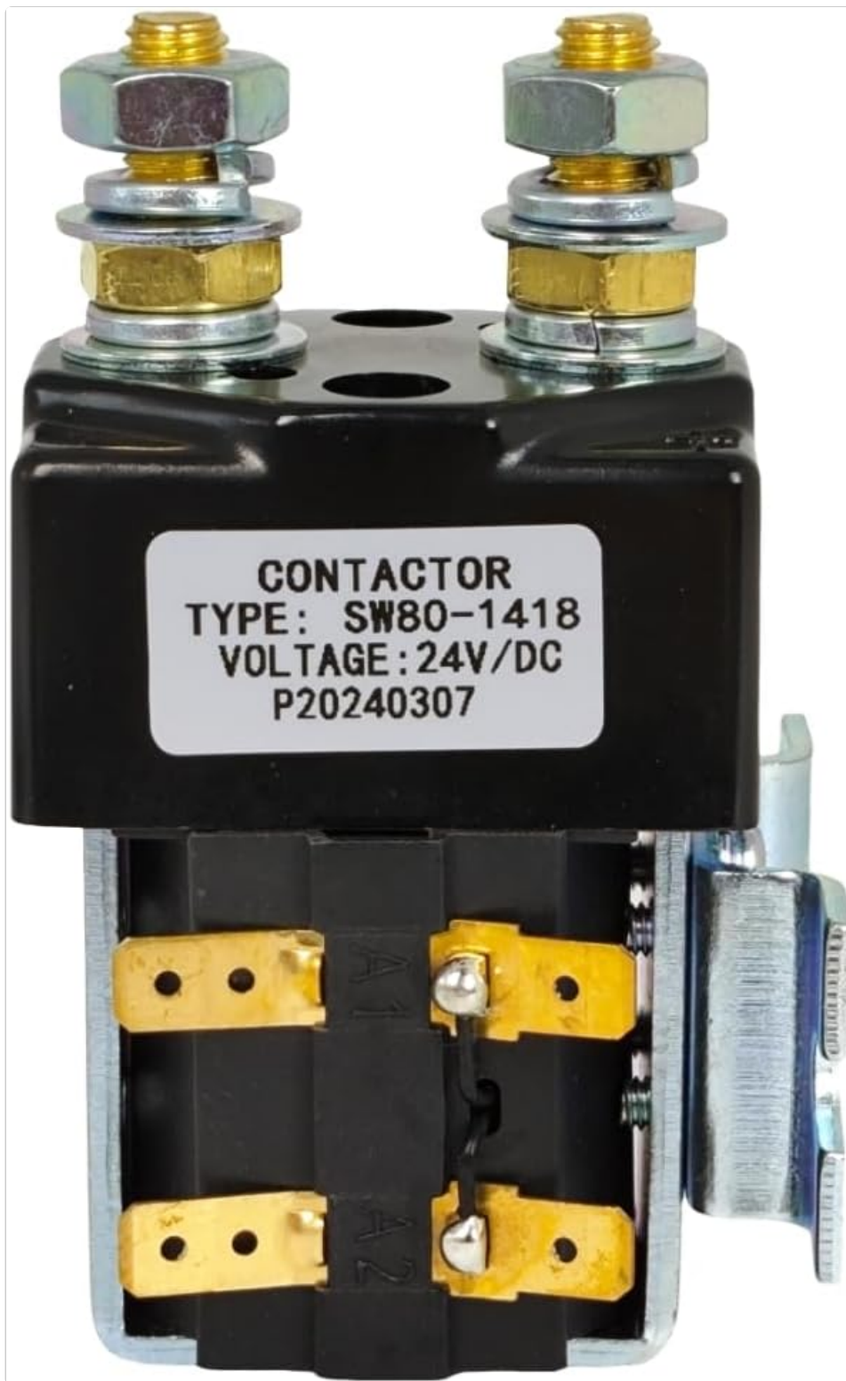
Figure 1: Front view of the solenoid with label and terminals. This image displays the main body of the solenoid, clearly showing the product label with model number SW80-1418 and voltage rating 24V/DC. The two large terminals for power connections are visible at the top, and the two smaller coil control terminals are at the bottom.
