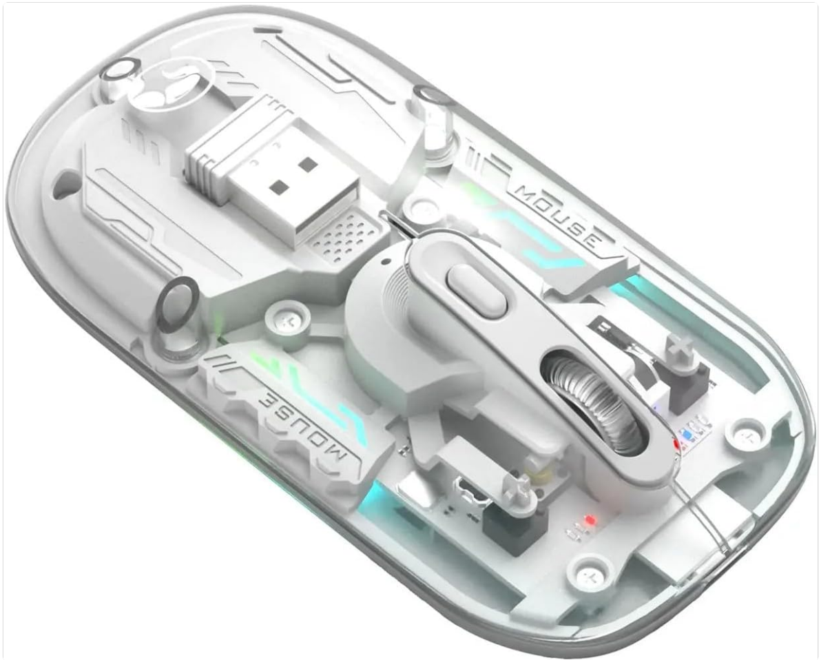
Figure 2: Angled view of the MARVO M808W Wireless Mouse, showcasing the scroll wheel, primary buttons, and the transparent design that reveals the internal electronics.
