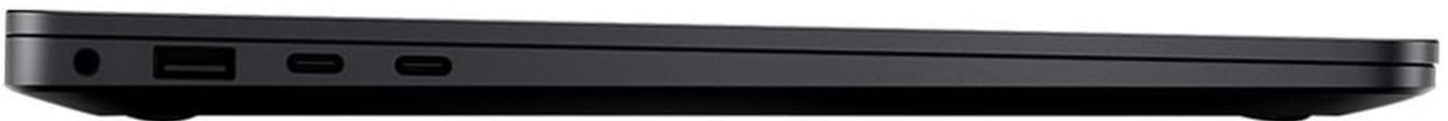
Figure 4: Side profile of the Surface Laptop, highlighting the USB ports and audio jack.
