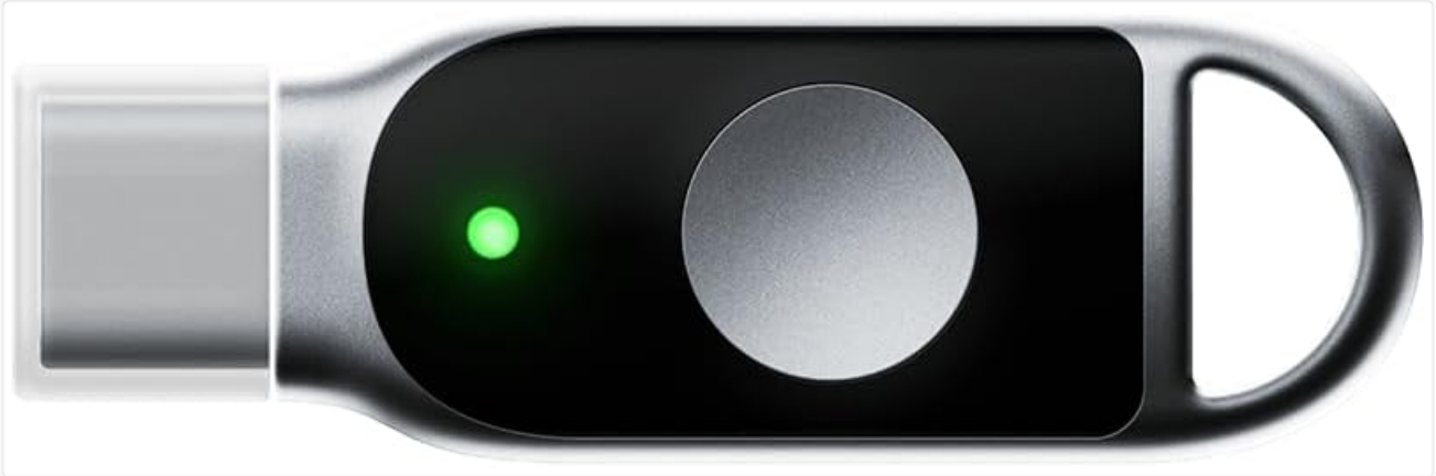
Figure 3.1: Front view of the FEITIAN K39 USB Security Key, showing the USB-C connector, the touch sensor, and a green indicator light, which signifies active status or successful authentication.
