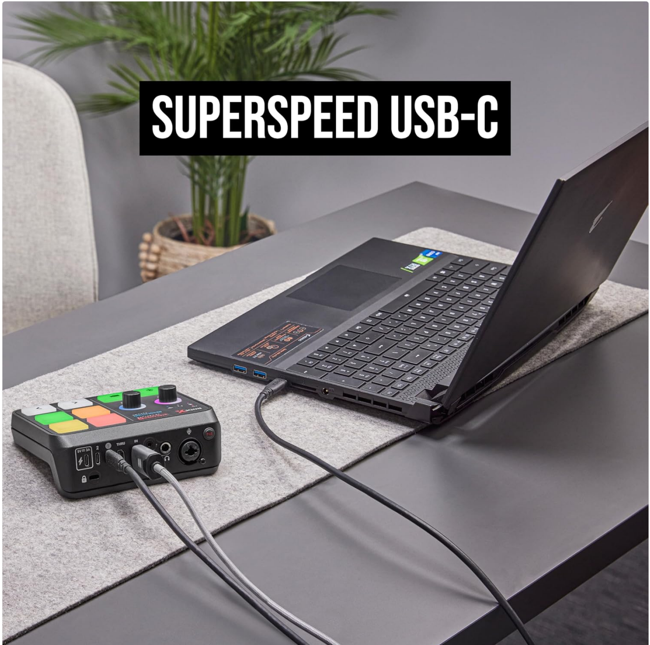
Image: The RØDE SC27 cable connecting a laptop to an audio interface, demonstrating its use for data transfer and power delivery.
