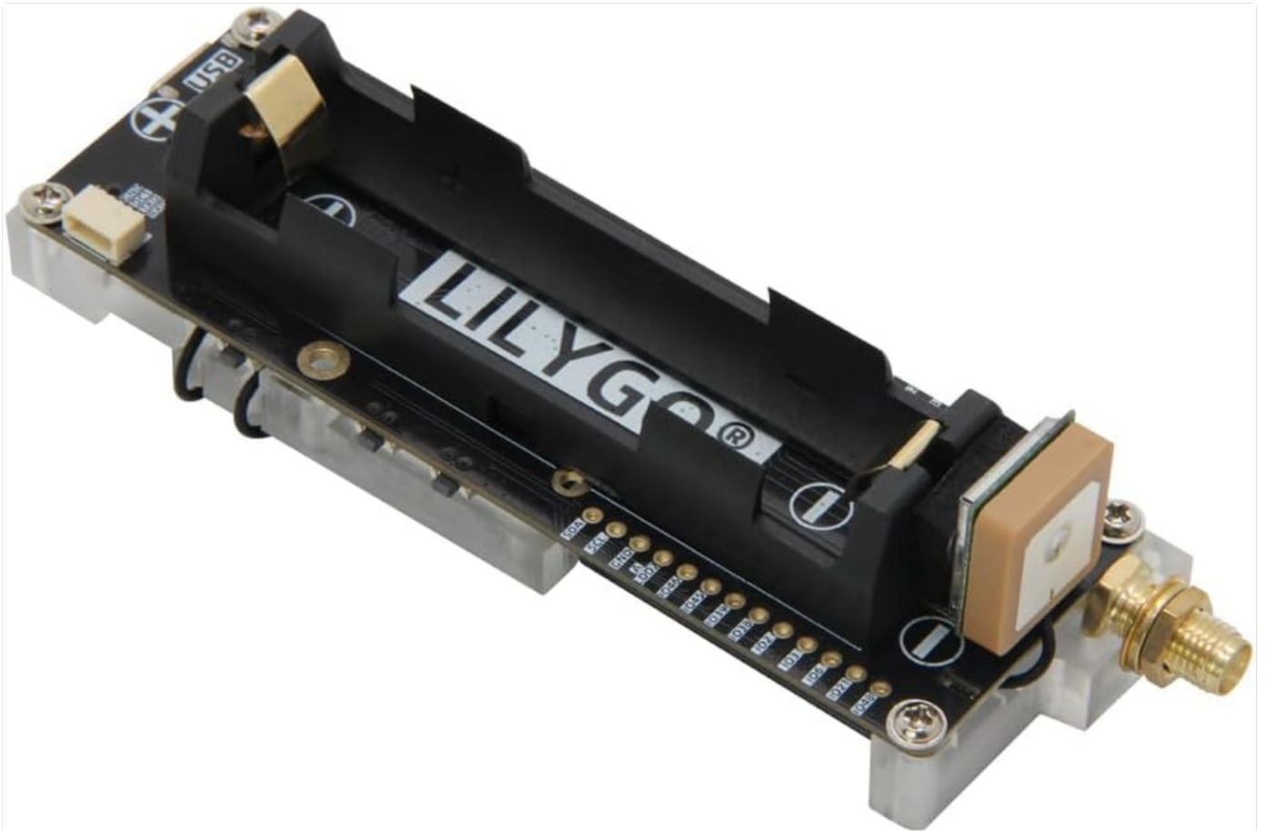
Figure 2.2.2: Back view of the LILYGO T-BeamSUPREME board, highlighting the 18650 battery holder and USB-C port.
