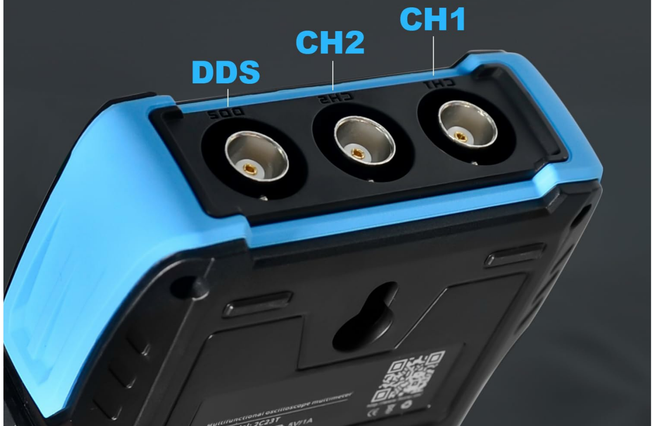
Image: Detail of the dual channel inputs (CH1, CH2) and the DDS signal generator output on the top of the device.
